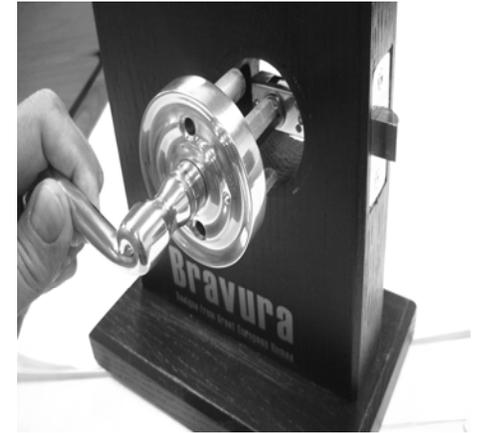
→6) Mounting screws are included for 1 3/8" thick and 1 3/4" thick doors. For 1 3/8" doors insert the two, shorter screws into the beveled holes of the non-public lock-half. During final tightening of these screws, support levers to hold them level. **DO NOT USE ELECTRIC DRILL!!** NOTE: to protect the finish on knobs during screw-installation, it is recommended that you keep them covered with their plastic shipping bag.
