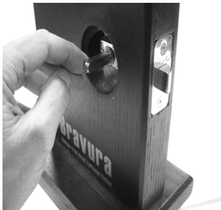
→ 3) Insert the spindle into the latch mechanism while depressing the button. The spindle is properly installed when the button pops-up on the opposite side of the latch, and the spindle is locked into place.
